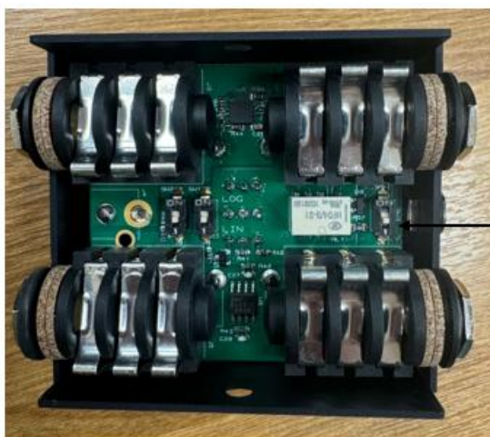
To enable CV mode – this switch must be in the on position
