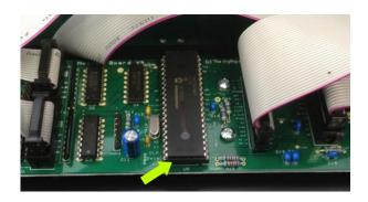
Step 4 - Lever out the chip gently with a pair of tweezers.
