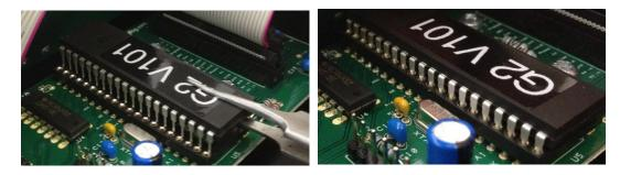
Step 7 – Follow steps 3 to 6 to update the Midi chip in the same way. The midi chip is located on the Motherboard to the left of where the foot switch cables are connected.
