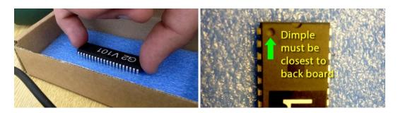
Step 6 - Using tweezers carefully apply even pressure and make sure the chip is fully installed. Make sure all the pins are inserted correctly.
