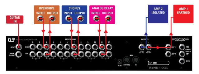
The way we'll mostly be using these effects loops is to connect our pedals. So the effects SEND from a G3/S loop is connected to the pedal INPUT, then the pedal OUTPUT is connected to the G3/S effects loop RETURN. So, if you are using a single amp or dual mono setup as per the above diagram you have 12 effects loops that you can use.
