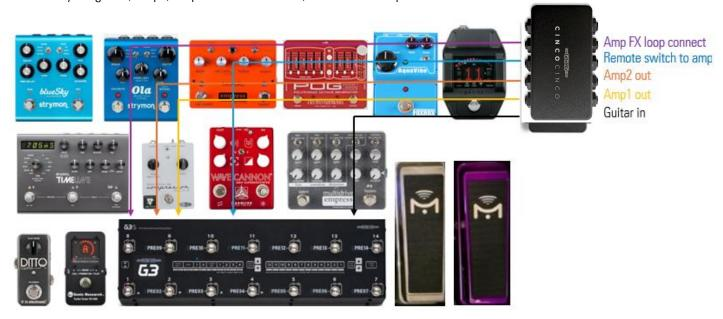
The example above uses four mono connections to link the guitar input, Amp 1, Amp 2, and the amp's remote switch to the G3. The 'Amp FX loop connect' requires a TRS (stereo) cable.
