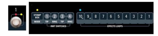
Now press the STOMP BOX MODE button. The yellow LED above the footswitch lights up telling you that preset 1 is set up in STOMP BOX MODE. The yellow led above the STOMP BOX MODE will also light up indicating that STOMP BOX has been selected for this sound. This preset is now set up in STOMP BOX MODE.
