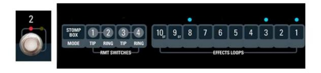
We want to ADD the delay from loop 10 ON TOP of this sound, but don't want to clear this sound. All we have to do is press preset number one which is set up in STOMP BOX MODE
