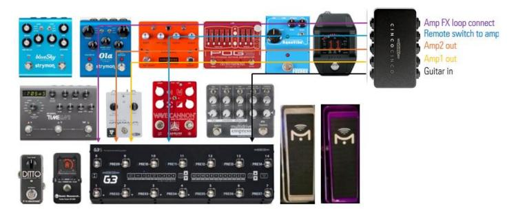
In the above example uses 4 mono connections to connect the Guitar input, Amp1, Amp2 and the Amp's Remote Switch to G3. The 'Amp FX loop connect' requires a TRS (stereo) cable.
